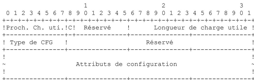
Figure 22 : Format de charge utile Configuration
